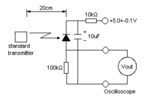
Fig.-3 Measuring System
